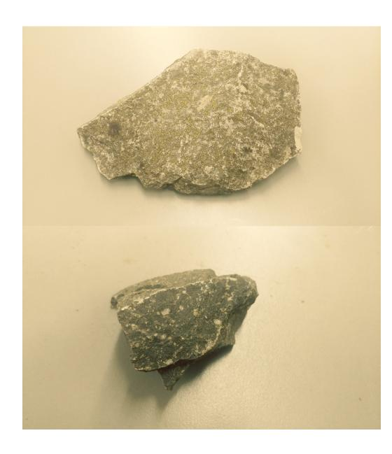
Basalt Samples from Collins Landslide Stockpile.
