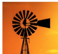
Figure 4: High solidity rotor
