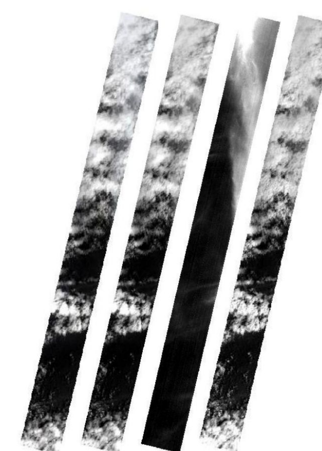
Right: Cirrus clouds as seen in visible, 870nm, 1.38µm, and 1.6µm bands.
